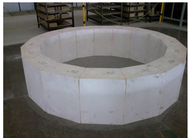
OPAL FURNACE LINED WITH MULLITE BLOCKS
